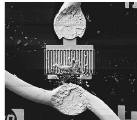
Fig. 6. Permanent damage of input transistor. Finger width is approximately 1 \mu\text{m} . Photo (SEM): C. Afzelius, FMV.
